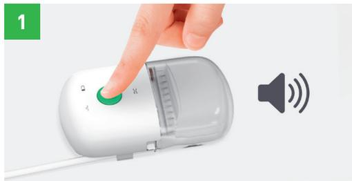
1 Pause the pump by pressing and holding the green start button and release after two (2) seconds. The pump will emit two beeps to confirm it is in a pause mode.
