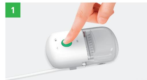
1 Pause the pump by pressing and holding the green start button and release after two (2) seconds. The pump will emit two beeps to confirm it is in a pause mode
